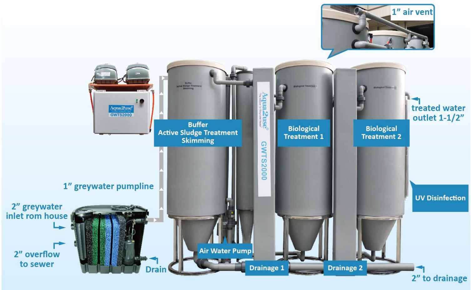
Figure 5. Inlet and outlet connections
