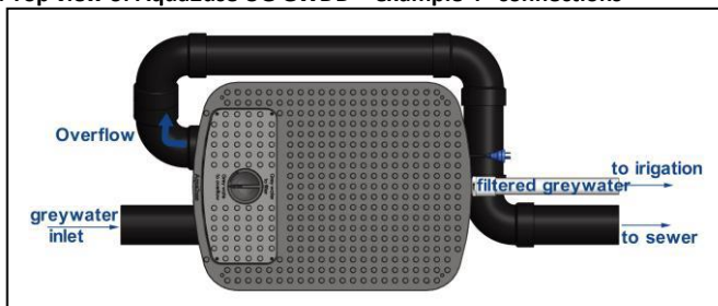
Fig. 3: Top view of Aqua2use UG GWDD – example 4” connections
